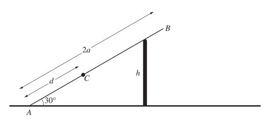
The diagram shows a ladder AB, of length 2a and mass m, resting in equilibrium on a vertical wall of height h. The ladder is inclined at an angle of  $30^{\circ}$  to the horizontal. The end A is in contact with horizontal ground. An object of mass 2m is placed on the ladder at a point C where AC = d.
